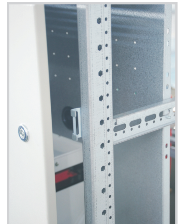
The frame adopts C type material, intensified the frame strength and decreased the error of connecting between each cabinet, better commonality, more convenient to install and maintain electrical components.
