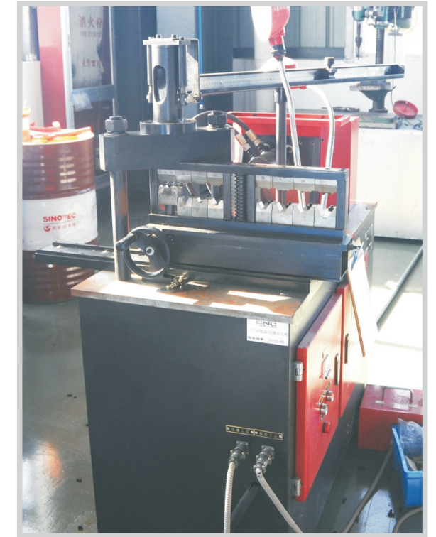
Adopt the dedicated machine to make the cable lug, ensure the reliability of cable lug and reduce the situation like cable lug fall off, lap resistance too big and virtual connection.
